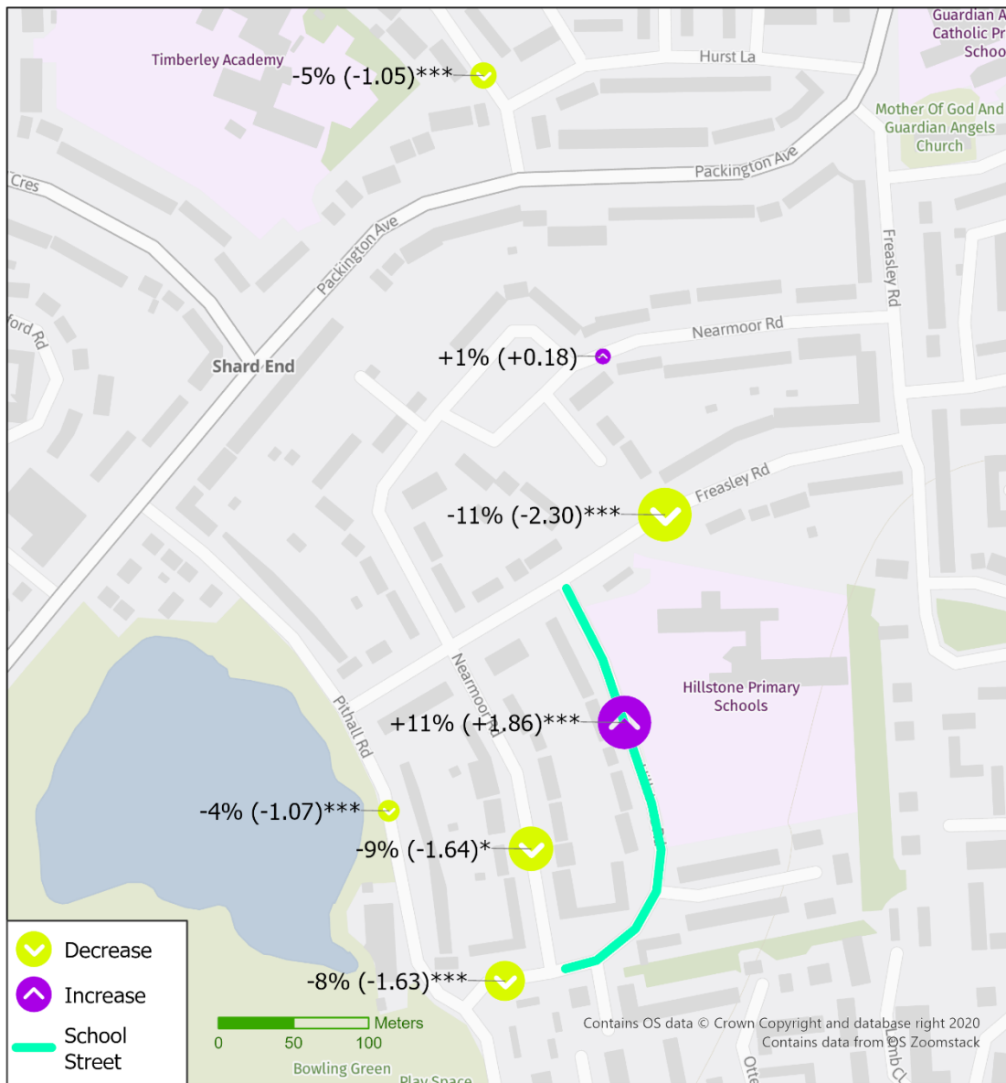
Figure 13: % (and numerical) change in average morning traffic speeds (08:00-09:00) between baseline and during intervention
