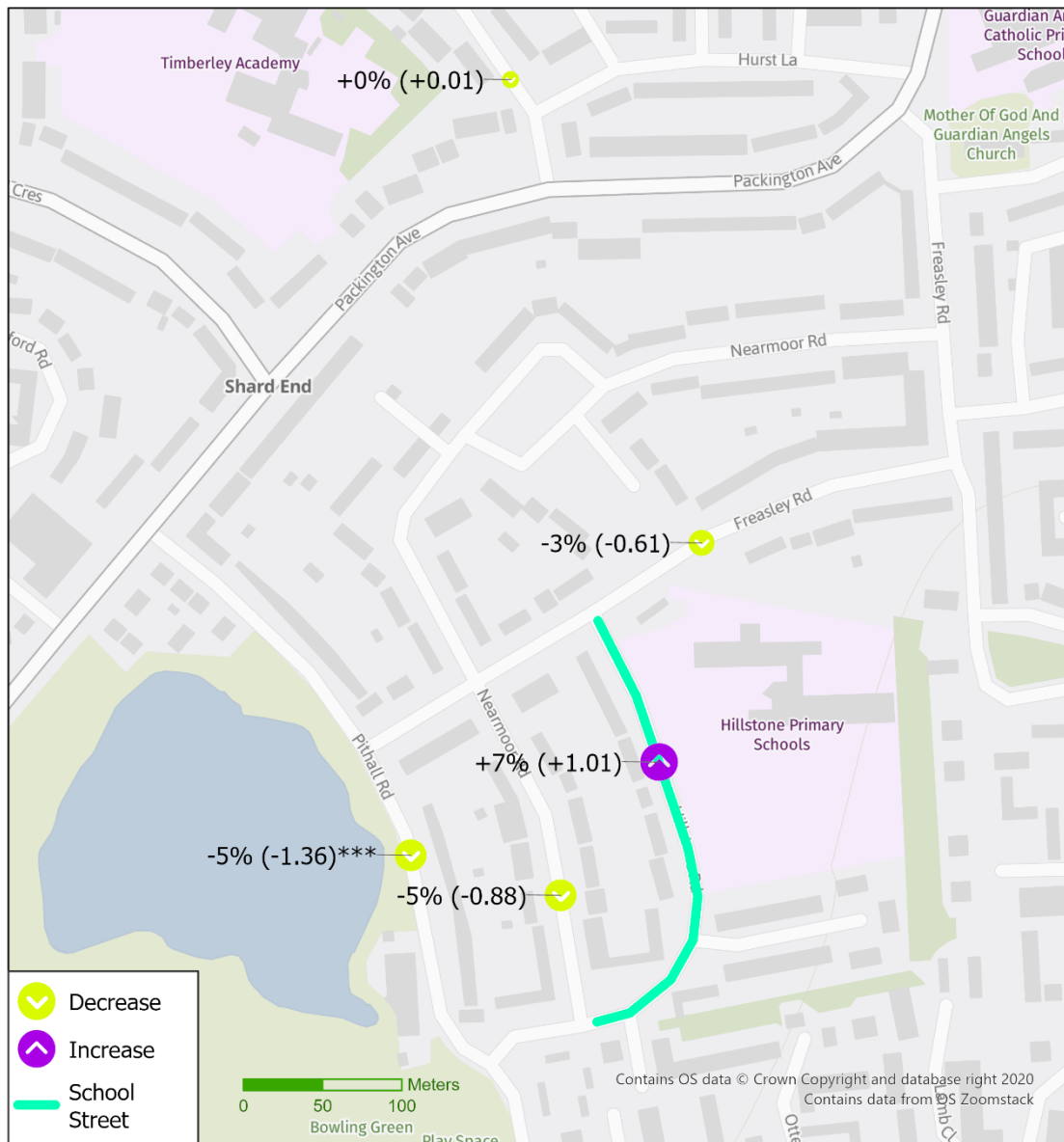
Figure 16: % (and numerical) change in average afternoon traffic speeds (14:45-15:45) between baseline and follow-up
