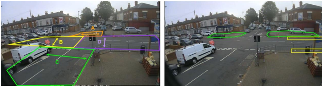
Figure 32: Markings for relevant behaviours at Somerville Video Location 1. Crossing points for pedestrians (left), and instances of drivers parking (right)
